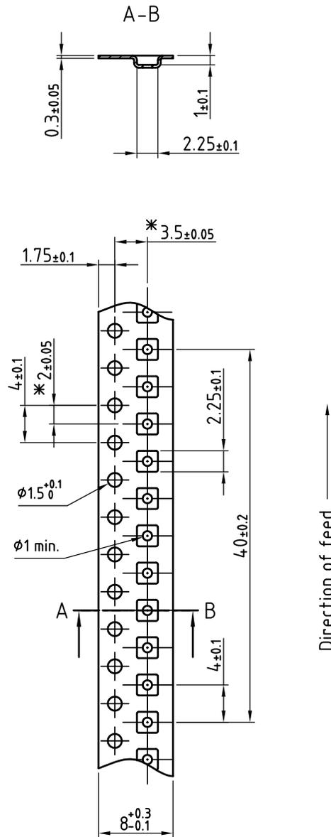
\* Measured from centerline of sprocket hole to centerline of pocket
