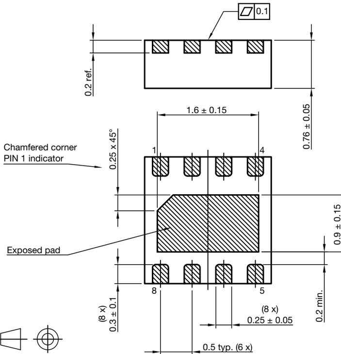
1. Coplanarity (0.1 mm) applies to the exposed pad as well as the exposed terminals.
