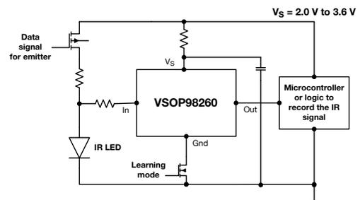
Recommended to minimize the connection distance between the IR LED and the input of the VSOP98260, and if possible to shield this connection to Gnd.
