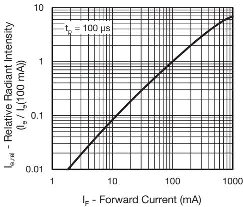
Fig. 4 - Relative Radiant Intensity vs. Forward Current
