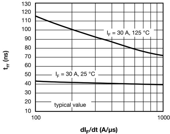
Fig. 7 - Typical Reverse Recovery vs.  $di_F/dt$
