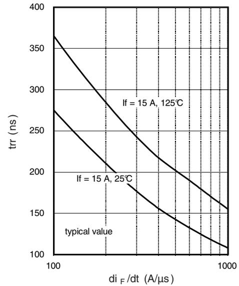
Fig. 7 - Typical Reverse Recovery vs.  $di_F/dt$
