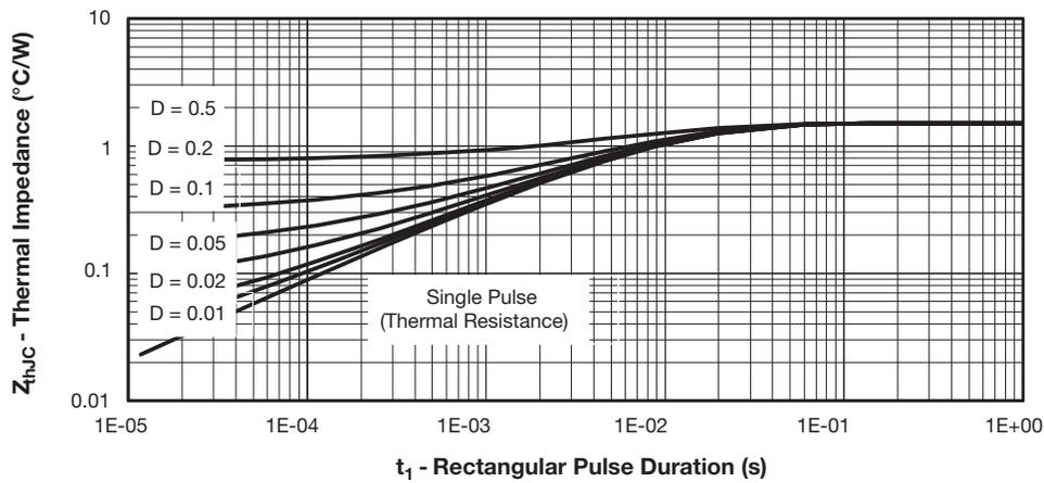
Fig. 4 - Max. Thermal Impedance  $Z_{thJC}$  Characteristics
