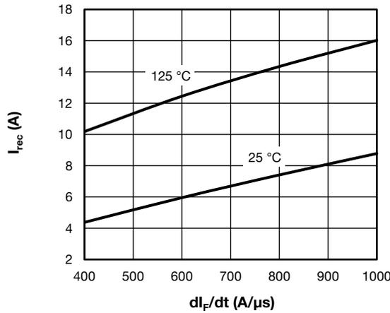
Fig. 9 - Typical Reverse Current vs.  $di_F/dt$
