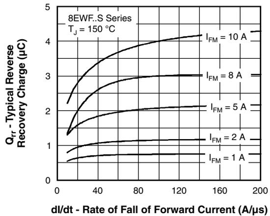
Fig. 11 - Recovery Charge Characteristics,  $T_J = 150\text{ °C}$
