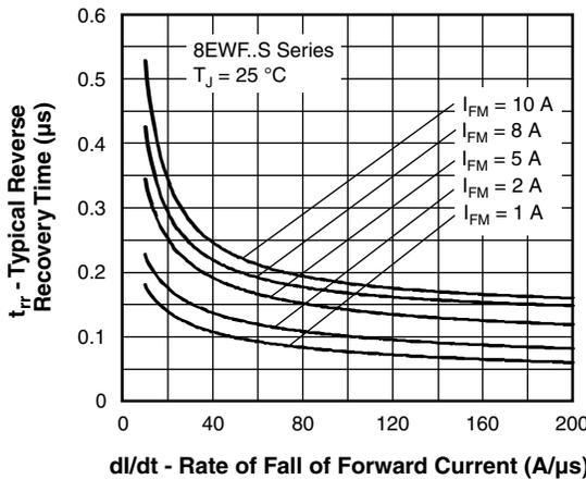
Fig. 8 - Recovery Time Characteristics,  $T_J = 25\text{ °C}$
