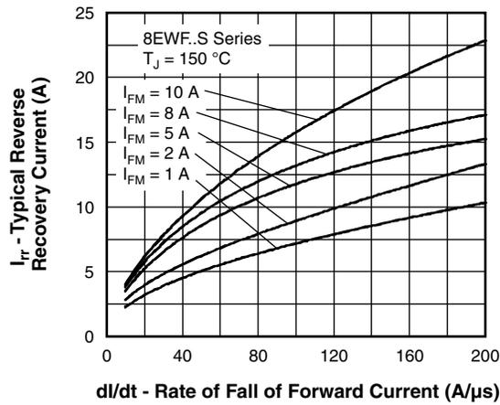
Fig. 13 - Recovery Current Characteristics,  $T_J = 150\text{ }^\circ\text{C}$
