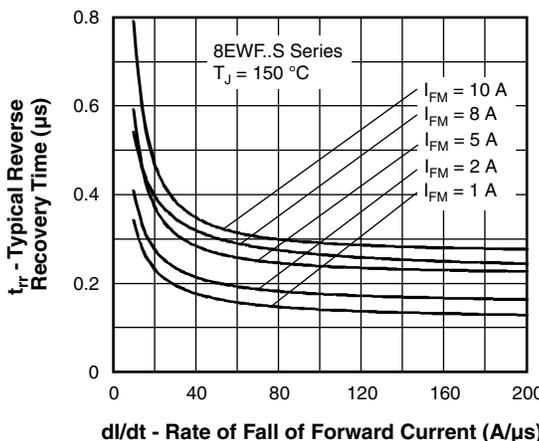
Fig. 9 - Recovery Time Characteristics,  $T_J = 150\text{ °C}$
