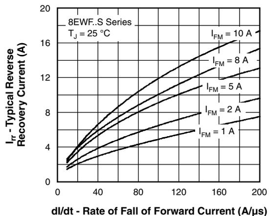
Fig. 12 - Recovery Current Characteristics,  $T_J = 25\text{ °C}$
