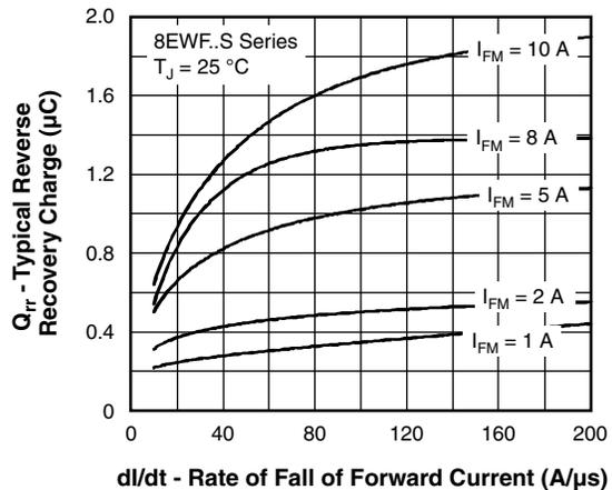
Fig. 10 - Recovery Charge Characteristics,  $T_J = 25\text{ °C}$
