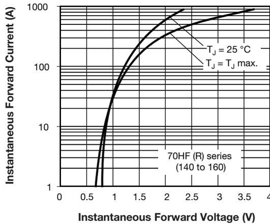
Fig. 13 - Forward Voltage Drop Characteristics
