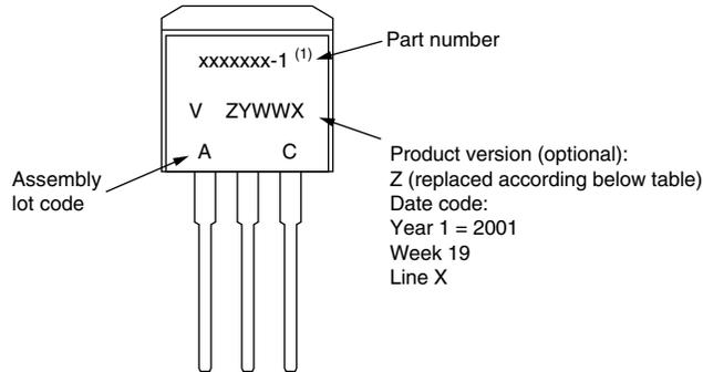
Example: This is a xxxxxx-1 <sup>(1)</sup> with assembly lot code AC, assembled on WW 19, 2001 in the assembly line "X"
