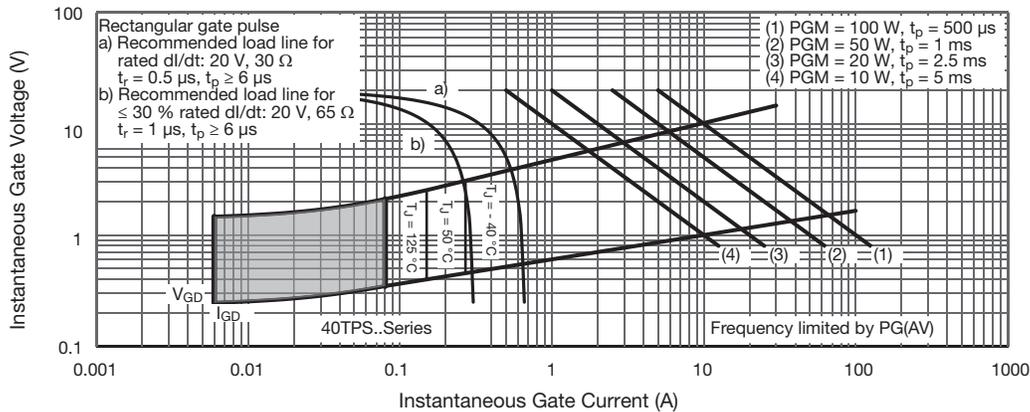
Fig. 8 - Gate Characteristics
