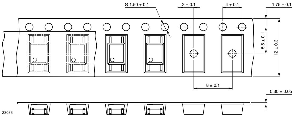
Fig. 14 - Tape and Reel Packaging (3000 pieces on reel)
