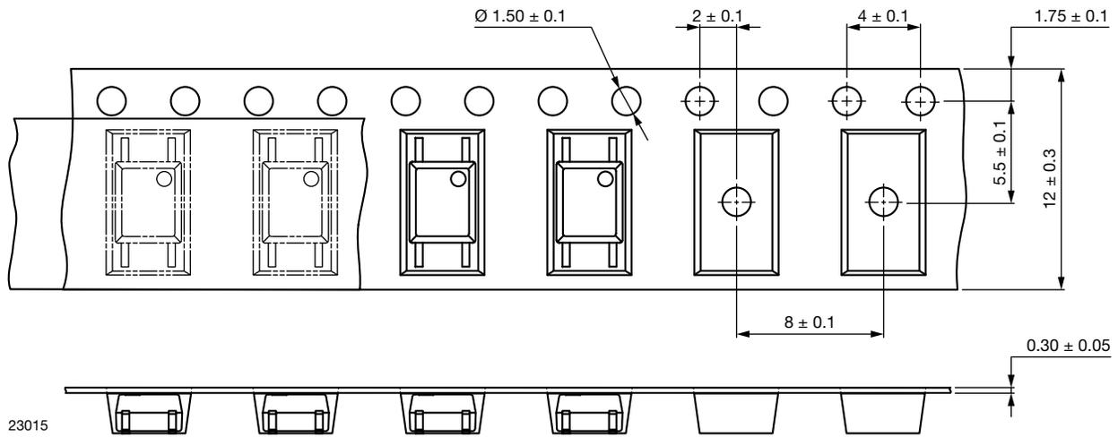
Fig. 13 - Tape and Reel Packaging (3000 pieces on reel)
