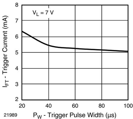
Fig. 10 - Trigger Current vs. Trigger Pulse Width
