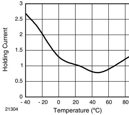
Fig. 10 - Normalized Holding Current vs. Temperature
