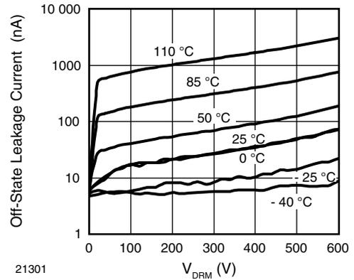
Fig. 7 - Off-State Leakage Current vs. Voltage
