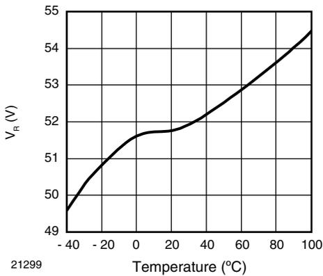
Fig. 5 - Diode Reverse Voltage vs. Temperature
