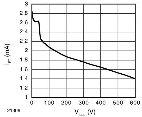
Fig. 12 - Trigger Current vs. V<sub>load</sub>
