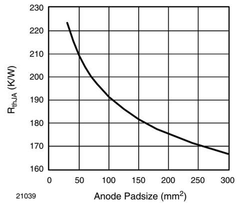
Fig. 5 - Thermal Resistance Junction Ambient vs. Anode Padsizes
