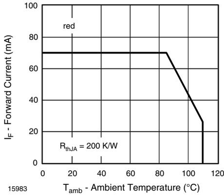
Fig. 1 - Maximum Permissible Forward Current vs. Ambient Temperature
