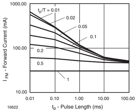
Fig. 2 - Forward Current vs. Pulse Length
