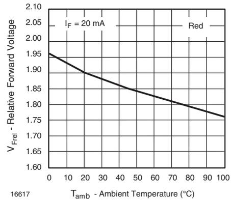
Fig. 8 - Forward Voltage vs. Ambient Temperature
