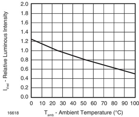
Fig. 7 - Relative Luminous Intensity vs. Ambient Temperature
