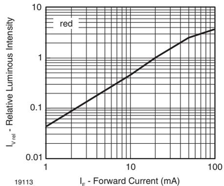
Fig. 6 - Relative Luminous Intensity vs. Forward Current
