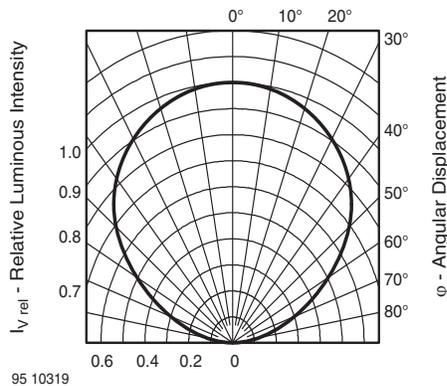
Fig. 3 - Relative Luminous Intensity vs. Angular Displacement
