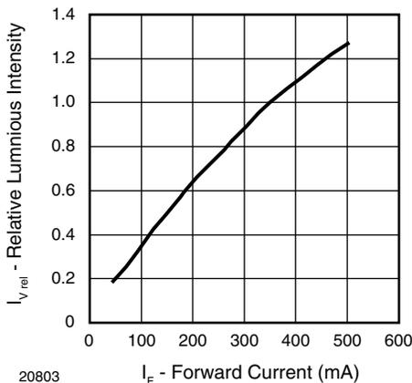
Fig. 2 - Relative Luminous Intensity vs. Forward Current
