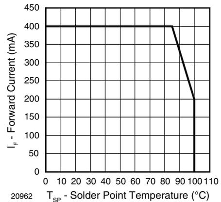
Fig. 3 - Forward Current vs. Solder Point Temperature
