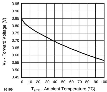
Fig. 7 - Forward Voltage vs. Ambient Temperature
