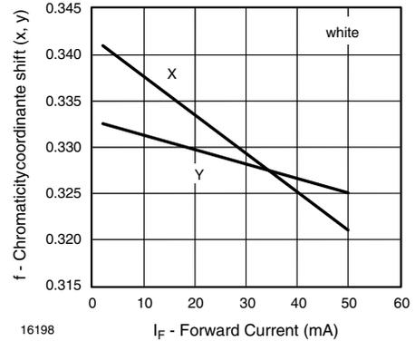
Fig. 8 - Chromaticity Coordinate Shift vs. Forward Current
