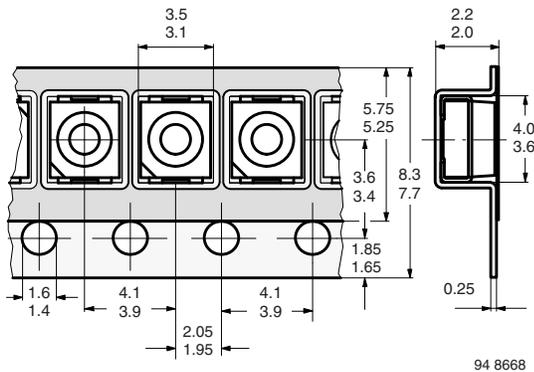
Fig. 10 - Tape Dimensions in mm for PLCC-2
