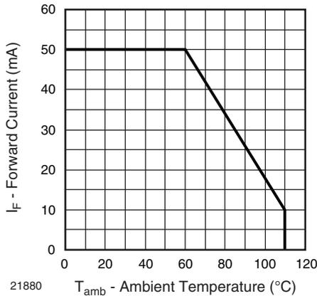
Fig. 1 - Forward Current vs. Ambient Temperature
