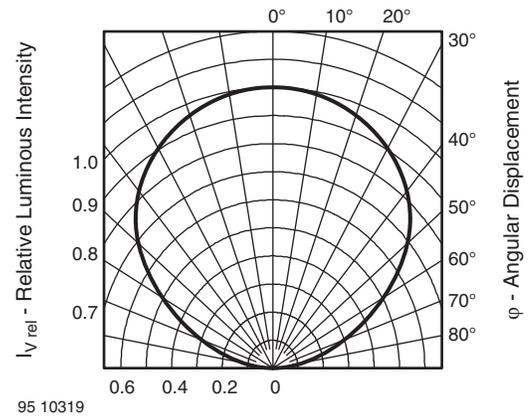
Fig. 5 - Relative Luminous Intensity vs. Angular Displacement
