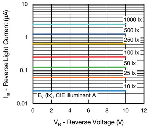
Fig. 3 - Reverse Light Current vs. Reverse Voltage
