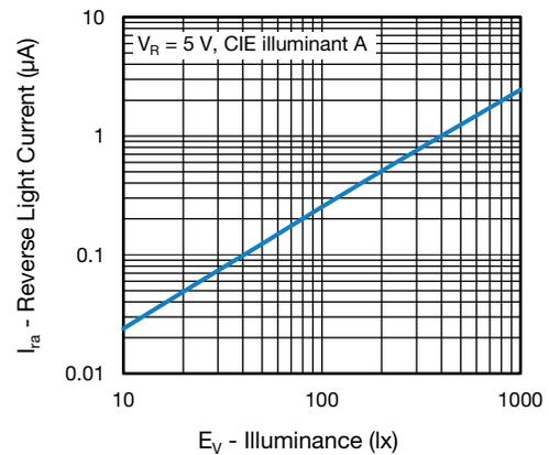
Fig. 2 - Reverse Light Current vs. Irradiance
