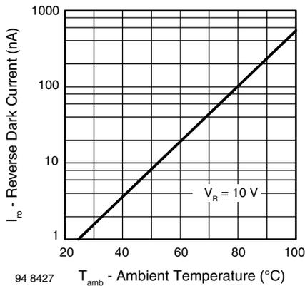
Fig. 1 - Reverse Dark Current vs. Ambient Temperature
