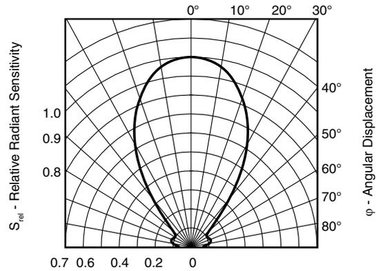
Fig. 6 - Relative Radiant Intensity vs. Angular Displacement
