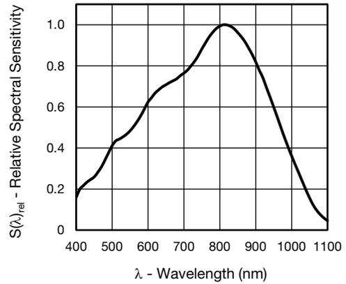
Fig. 6 - Relative Spectral Sensitivity vs. Wavelength
