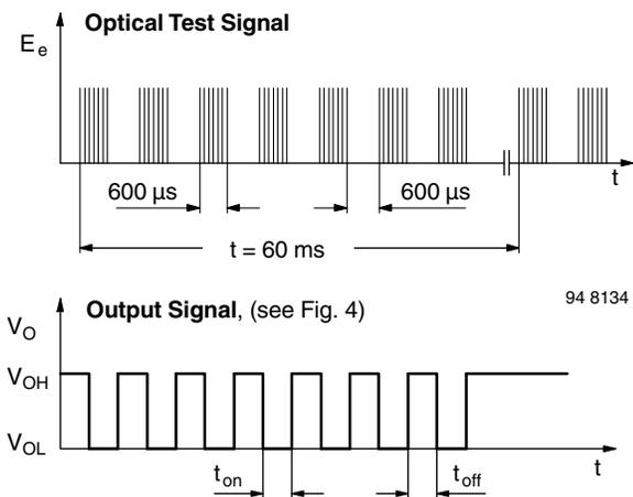
Fig. 3 - Test Signal
