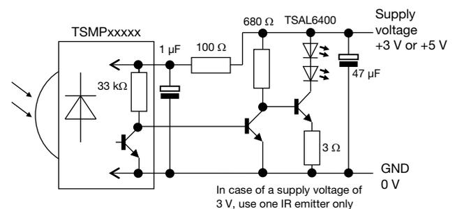
Recommended circuit for best sensitivity in repeater applications. It limits the output voltage swing  $V_o$  to about 0.7 V in order to avoid internal coupling.
