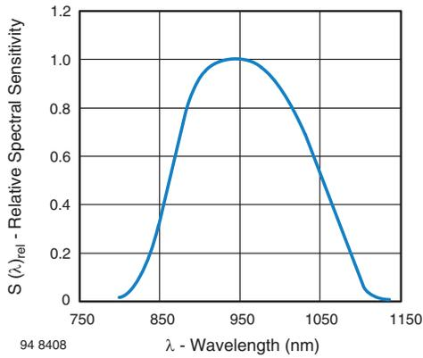
Fig. 3 - Relative Spectral Sensitivity vs. Wavelength
