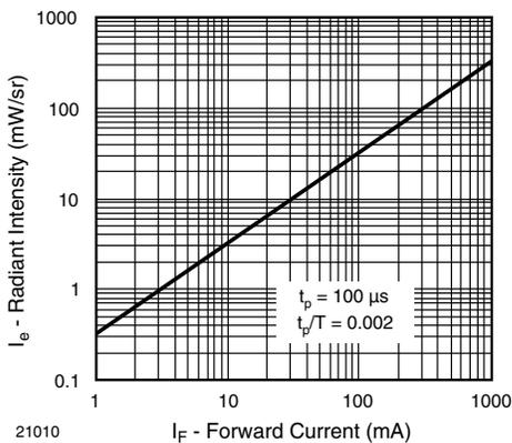
Fig. 5 - Radiant Intensity vs. Forward Current
