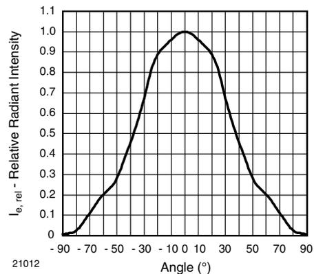
Fig. 8 - Relative Radiant Intensity vs. Angular Displacement
