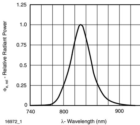
Fig. 7 - Relative Radiant Power vs. Wavelength
