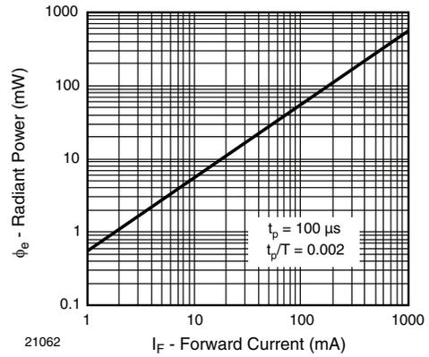
Fig. 6 - Radiant Power vs. Forward Current
