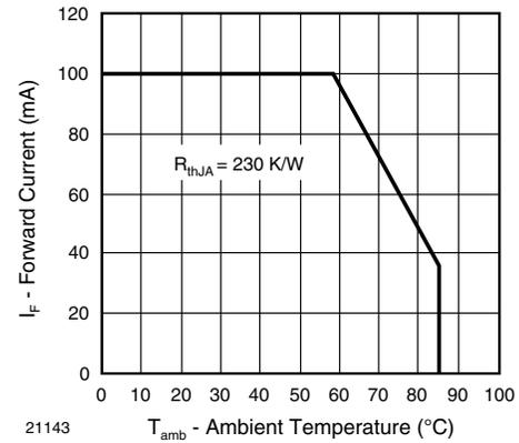
Fig. 1 - Forward Current Limit vs. Ambient Temperature
