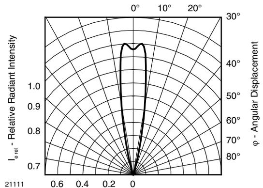
Fig. 7 - Relative Radiant Intensity vs. Angular Displacement
