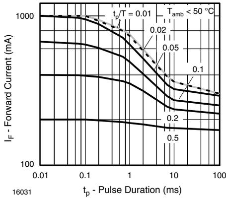
Fig. 2 - Pulse Forward Current vs. Pulse Duration
