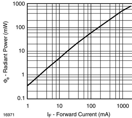
Fig. 5 - Radiant Power vs. Forward Current
