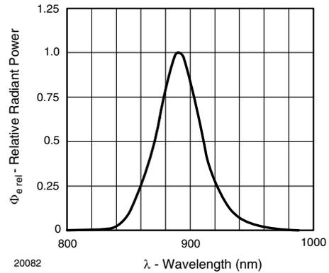
Fig. 7 - Relative Radiant Power vs. Wavelength
