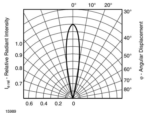
Fig. 8 - Relative Radiant Intensity vs. Angular Displacement
