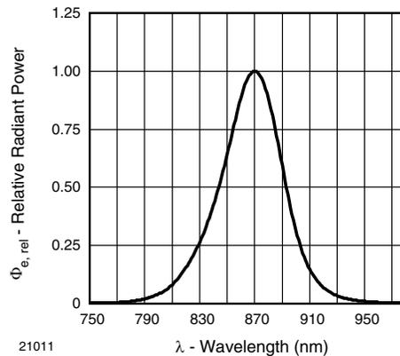
Fig. 6 - Relative Radiant Power vs. Wavelength
