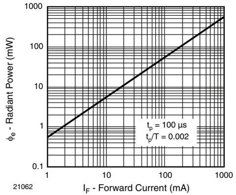
Fig. 5 - Radiant Power vs. Forward Current
