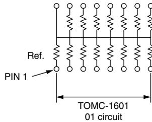
The 01 circuit provides 15 nominally equal resistors, each connected between a common lead (16) and a discrete PC board pin.
