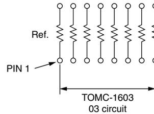
The 03 circuit provides a choice of 8 nominally equal resistors with each resistor isolated from all others and wired directly across.
