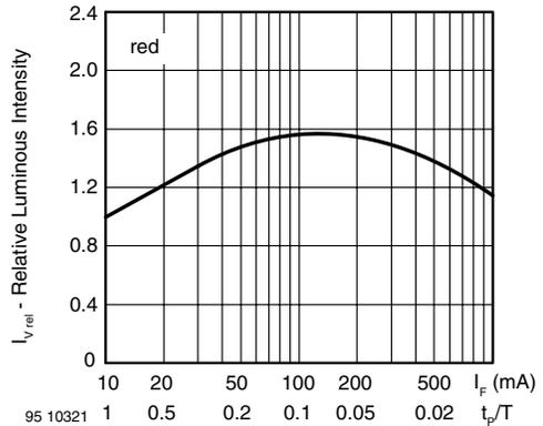
Figure 7. Rel. Luminous Intensity vs. Forw. Current/Duty Cycle
