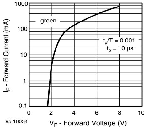
Fig. 14 - Forward Current vs. Forward Voltage
