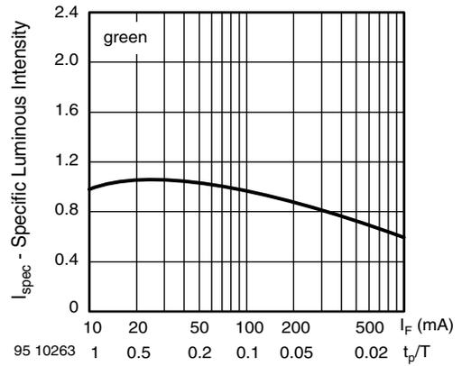
Fig. 16 - Specific Luminous Intensity vs. Forward Current
