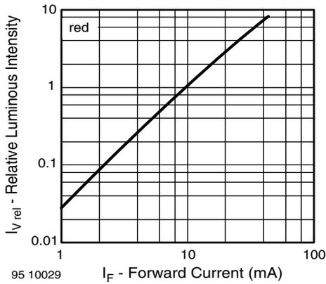
Fig. 7 - Relative Luminous Intensity vs. Forward Current
