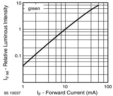
Fig. 17 - Relative Luminous Intensity vs. Forward Current
