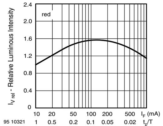
Fig. 6 - Relative Luminous Intensity vs. Forward Current/Duty Cycle
