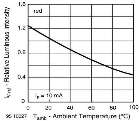
Fig. 5 - Relative Luminous Intensity vs. Ambient Temperature
