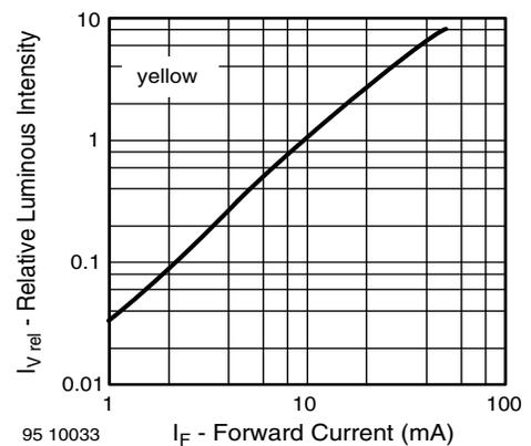
Fig. 12 - Relative Luminous Intensity vs. Forward Current
