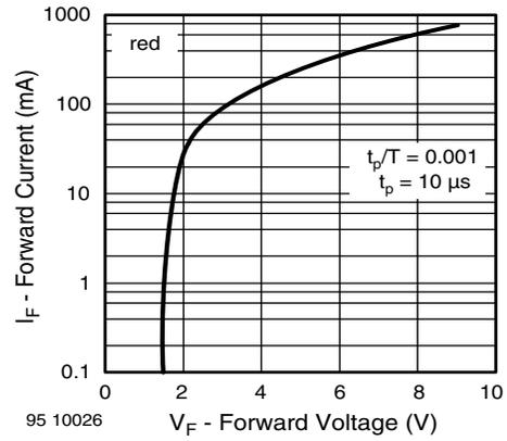
Fig. 4 - Forward Current vs. Forward Voltage
