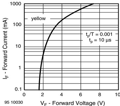
Fig. 9 - Forward Current vs. Forward Voltage
