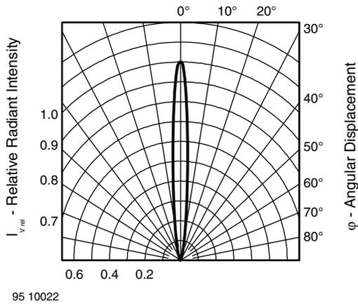
Fig. 2 - Relative Luminous Intensity vs. Angular Displacement
