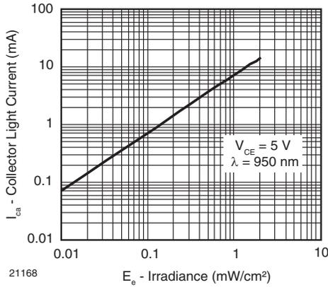
Fig. 4 - Collector Light Current vs. Irradiance
