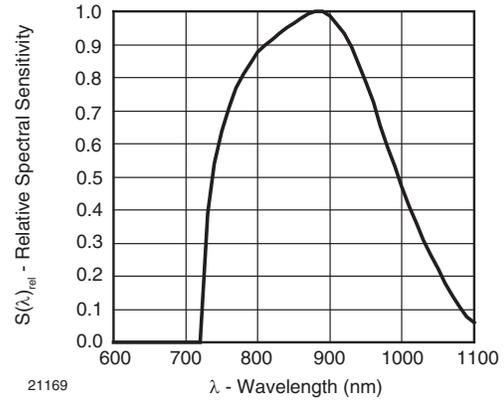
Fig. 7 - Relative Spectral Sensitivity vs. Wavelength
