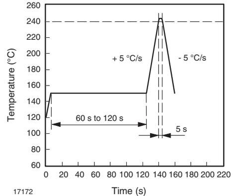
Fig. 9 - Lead Tin (SnPb) Reflow Solder Profile
