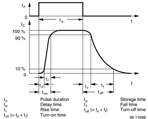
Fig. 5 - Switching Times
