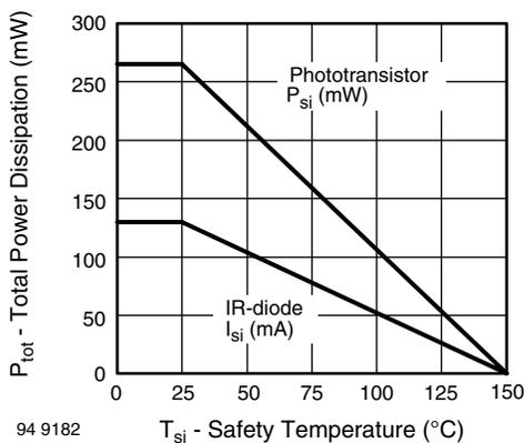
Fig. 1 - Derating Diagram
