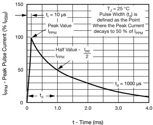
Fig. 3 - Pulse Waveform
