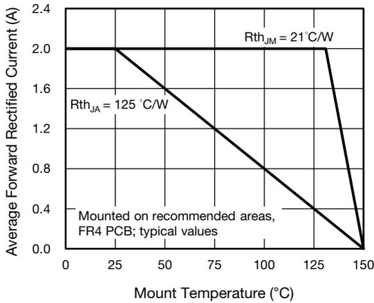
Fig. 1 - Typical Forward Current Derating Curve
