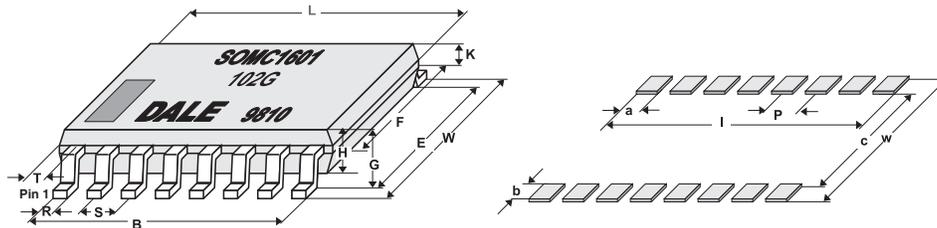
**SOLDER PAD DIMENSIONS** in millimeters
