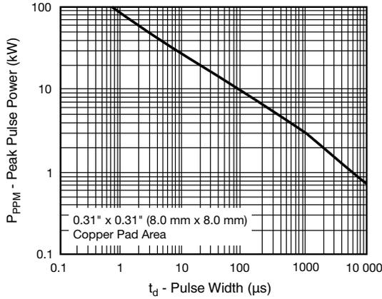
Fig. 1 - Peak Pulse Power Derating Curve
