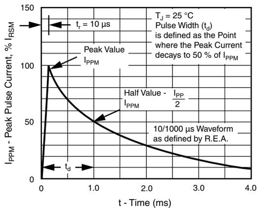
Fig. 3 - Pulse Waveform
