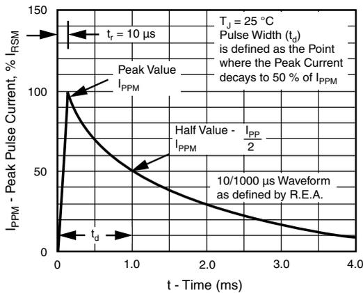
Fig. 3 - Pulse Waveform
