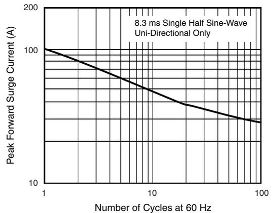
Fig. 6 - Maximum Non-Repetitive Peak Forward Surge Current
