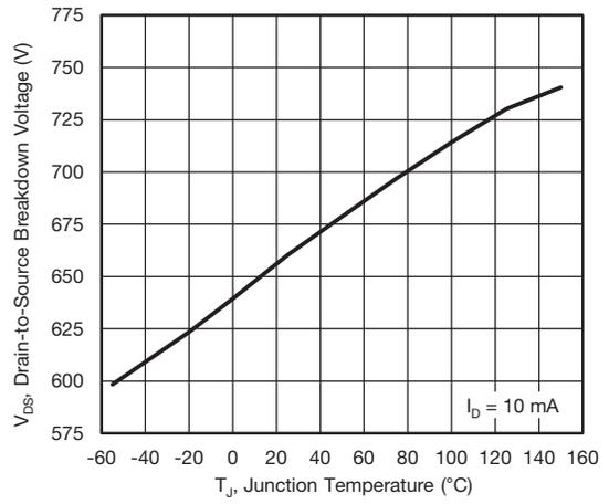
**Fig. 11 - Typical Drain-to-Source Voltage vs. Temperature**
