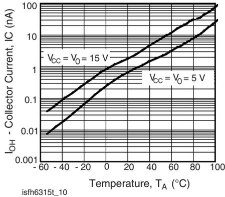
Fig. 9 - Logic High Output Current vs. Temperature
