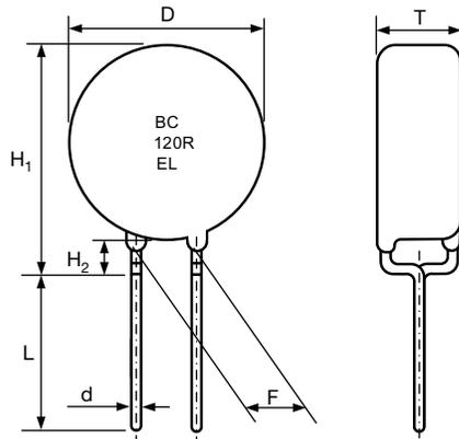
**COMPONENT DIMENSIONS** in millimeters
