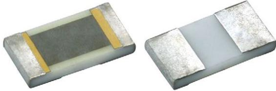
PHP series chip resistors are designed with enlarged backside terminations to reduce the thermal resistance between the topside resistor layer and the solder joint on the end users circuit board.
