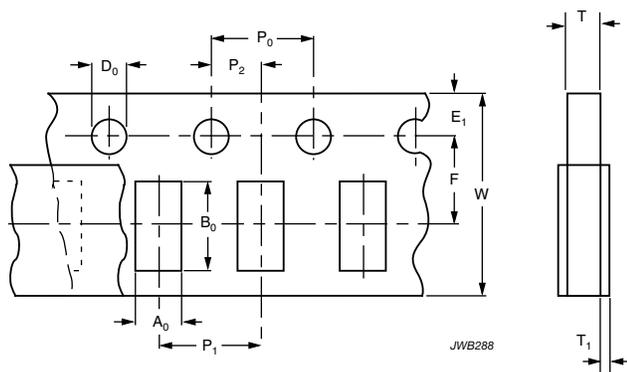
**DIMENSIONS OF PAPER TAPE** in millimeters
