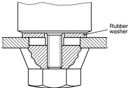
Fig. 6 - Insulated mounting
