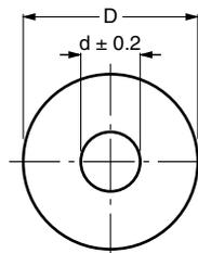
Fig. 8 - Rubber washer; thickness 2 mm
