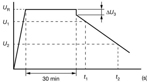
Fig. 4 - Voltage Diagram for Capacitance Measurement
