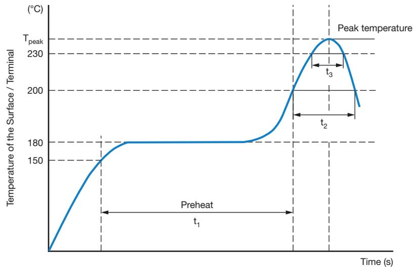
Fig. 4 - Maximum temperature load during reflow soldering
