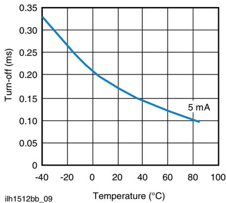
Fig. 9 - Form A Typical Turn-Off vs. Temperature
