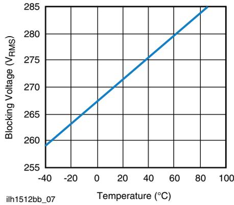
Fig. 7 - Form A Typical Blocking Voltage vs. Temperature
