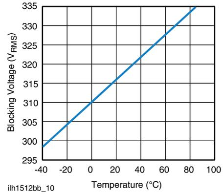
Fig. 10 - Form B Typical Blocking Voltage vs. Temperature
