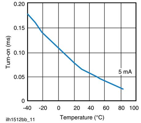
Fig. 11 - Form B Typical Turn-On vs. Temperature
