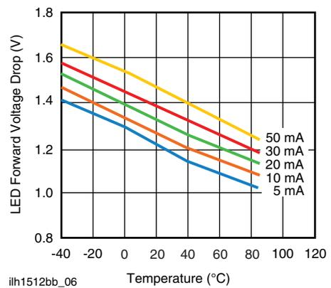
Fig. 6 - Typical LED Forward Voltage Drop vs. Temperature
