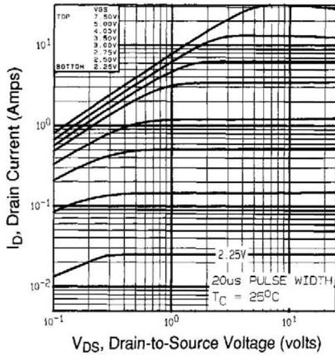
Fig. 1 - Typical Output Characteristics,  $T_C = 25\text{ }^\circ\text{C}$
