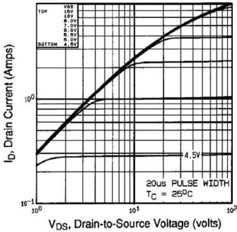
Fig. 1 - Typical Output Characteristics,  $T_C = 25\text{ }^\circ\text{C}$
